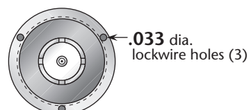
Coupling nut detail
