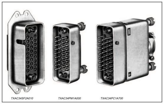
The TXAC Series was designed for external installation specifically for the industrial/ commercial customer in high temperature, rough service applications. This series features the same military-type anodized aluminum hoods, rugged polyester thermoplastic insulators, screw-machine removable contacts, guide and jack hardware, and protective, anodized aluminum shells as the XAC Series. These features make this Series suitable for chassis mounting, bulkheads, or any outside surface equipment.
