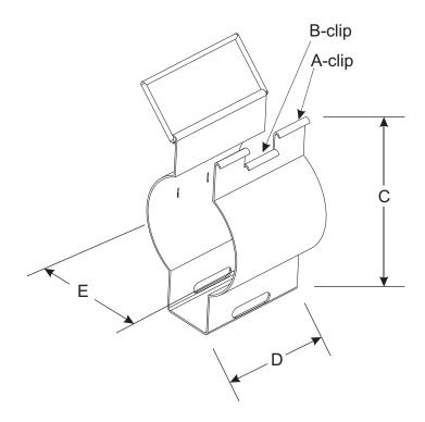
The dual-clip feature will allow the hanger to support a variety of brands of coaxial cable.
