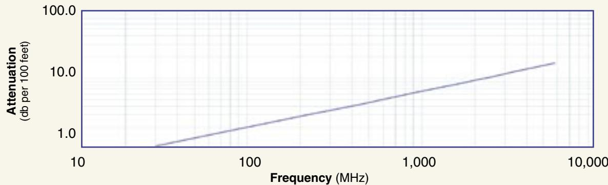
Calculate Attenuation =  $(0.200179) \cdot \sqrt{F \text{MHz}} + (0.000183) \cdot F \text{MHz}$  (interactive calculator available at [http://www.timesmicrowave.com/cable\\_calculators](http://www.timesmicrowave.com/cable_calculators))
