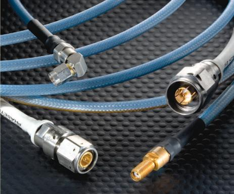
PhaseTrack™ 210 cable assemblies are designed for applications demanding minimal change over temperature. All PhaseTrack cables use proprietary TF4™ dielectric that does not have the abrupt shift in the phase that occurs with solid or tape wrapped PTFE based products under normal room ambient conditions.
