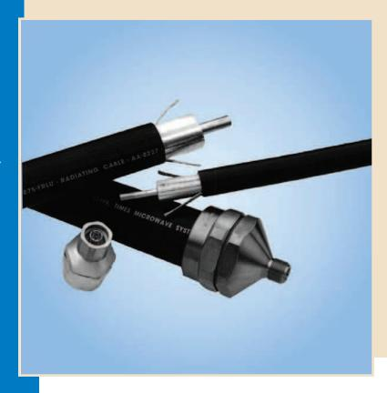
nu-TRAC TRC-1250 triaxial antenna cable is designed to provide controlled coverage in areas where RF propagation from a point source antenna is ineffective. Examples of common installations are subways, tunnels, ships, and metal framed buildings. The cable can function both as a transmit and receive antenna over a broad range of frequencies. The unique triaxial design allows for the cable to be mounted directly to a wall, thus eliminating cable standoffs and facilitating easy installation.
