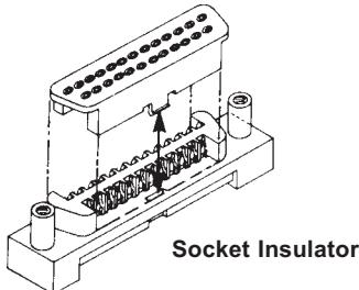
Individual contacts can be removed and replaced with a simple hand tool. See page CP/51 for tool part numbers.
