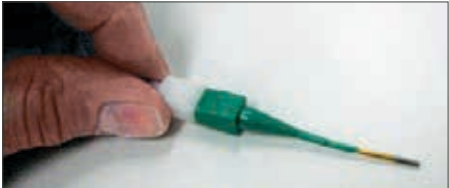
Plastic tool with contact in proper position.
